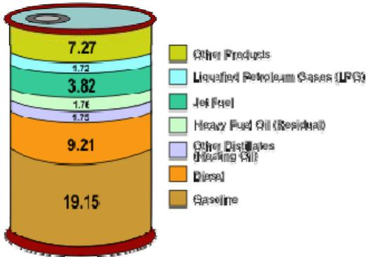
**Products from a Barrel of Crude Oil, Gallons<sup>8</sup>**
